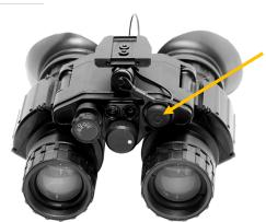
Momentary IR-On Button Allows to Instantly Engage IR Illuminator to Quickly Illuminate a Certain Area or Send a Morse-Code Signal to a Team Member.
